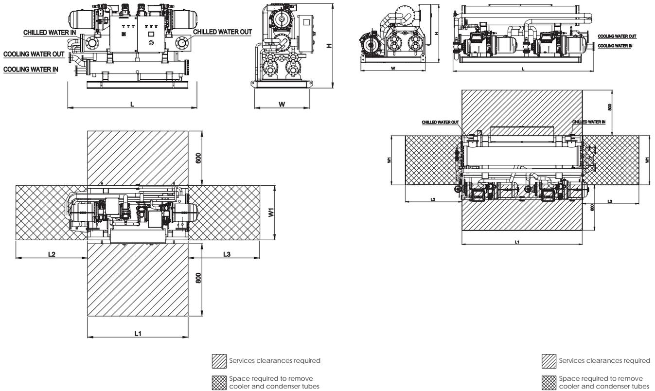
Dimensions: vertical type single compressor units
