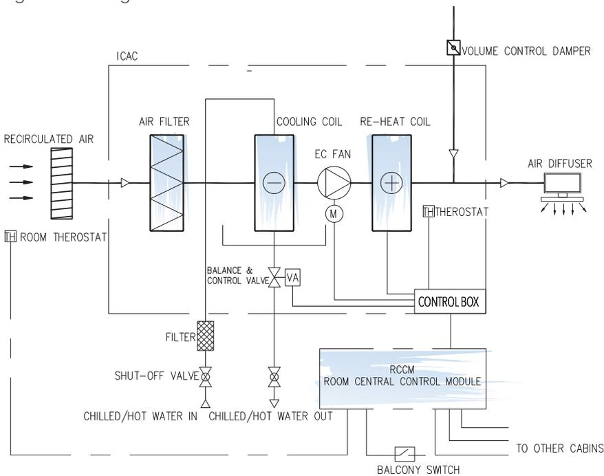
Fig. 2 The principle of the cabin air conditioner system, vertical ICAC
