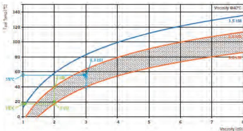
Depending on installation the viscosity of MGO should be min.2-3 cSt when entering the engines.
