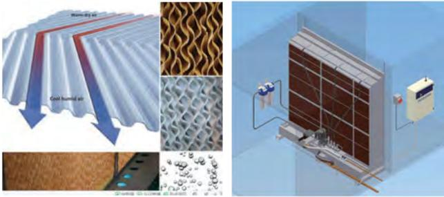
Evaporative humidifiers provide humidification and cooling without any aerosols in the AHU. This means they can be situated in short section lengths without the risk of wetting on bends. As minerals left behind after evaporation are regularly flushed to drain, service requirements are considerably less than steam humidification.
