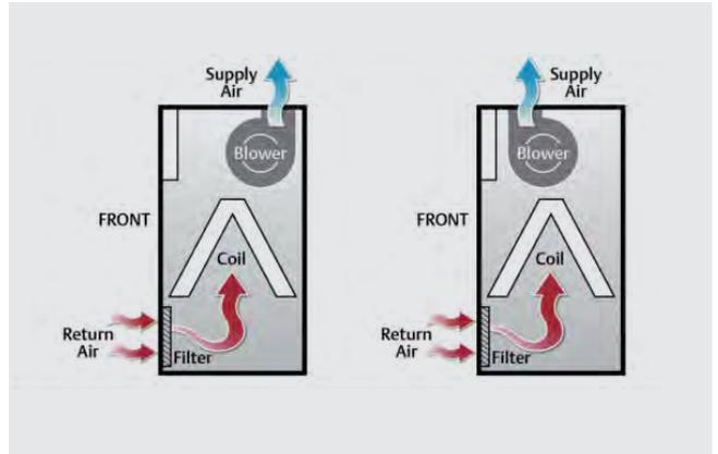
Fig.2 Down-flow configurations, bottom or under floor supply with EC fan
