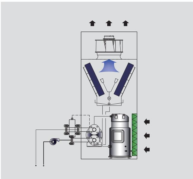
Water cooled down-flow configuration
