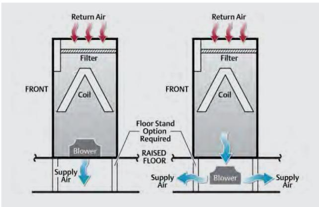
Fig.5 Up-flow configurations rear-return with forward-curved blowers
