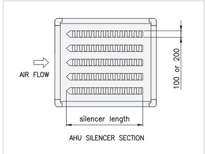
Absorption silencer consist of functions with lengths 600, 900,1200mm equipped with a number of vertical sound-absorbing baffles 100, or 200mm thick.
