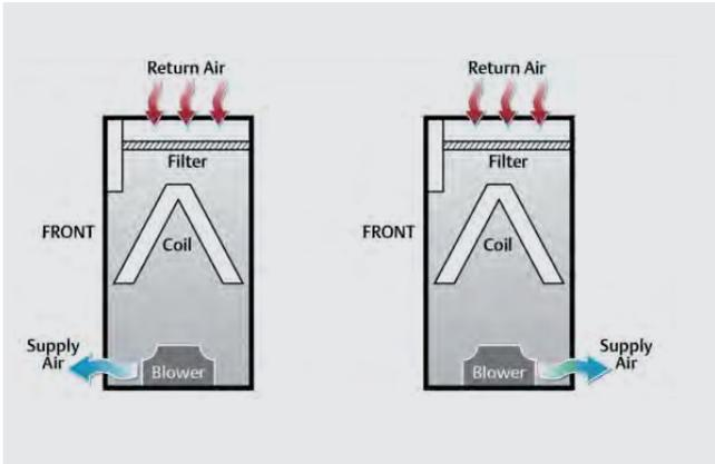
Fig.4 Up-flow configurations, front-return with forward-curved blowers
