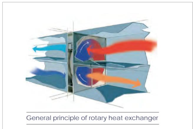
Rotary heat exchangers belong to the group regenerative heat exchangers. Rotor movement means that exhaust air and supply air pass the rotor medium alternately. A major proportion of the energy in the exhaust air is transferred to the supply air via the rotor medium. Thanks to the alternating airflow direction, the rotor is self-cleaning and frost proof to a large extent.
