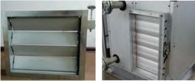
As standard, the air handling unit fitted with fresh air and return air shut-off dampers for air flow balance. The standard dampers blade are made of extruded aluminum and supported on nylon bushings in a sheet steel frame. The shafts are made of stainless steel. Other combinations of material are available on request.
