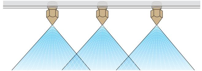
A compressed air and water humidifier offers guaranteed evaporation of the moisture into the atmosphere without any potential risk of drips. By forcing the water to mix with the air under pressure the sprays produced are rapidly absorbed and highly directional.
