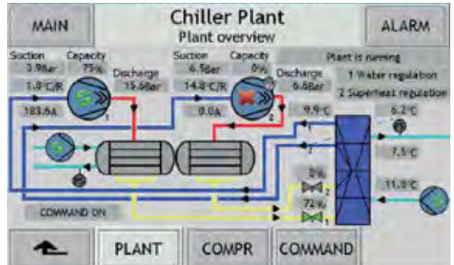
Sequencer panel with common chilled water (inlet/outlet) control
