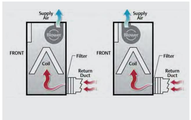
Fig. 3 Up-flow configurations with EC fan in a plenum, supply air exits the front or rear only
