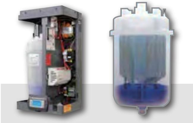
The operation of immersed electrode humidifiers is based on a very simple physical principle. As common drinking water contains a certain quantity of dissolved mineral salts, and is consequently slightly conductive, applying a voltage to metal electrodes immersed in the water until producing steam (Joule effect). The quantity of steam produced is proportional to the electric current, which is in turn proportional to the water level.
